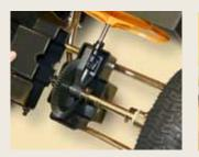
**Self-Lubricating Bearings** The axle and wheel bearings/ bushings provide self-lubrication with excellent wear and load-carrying performance.
